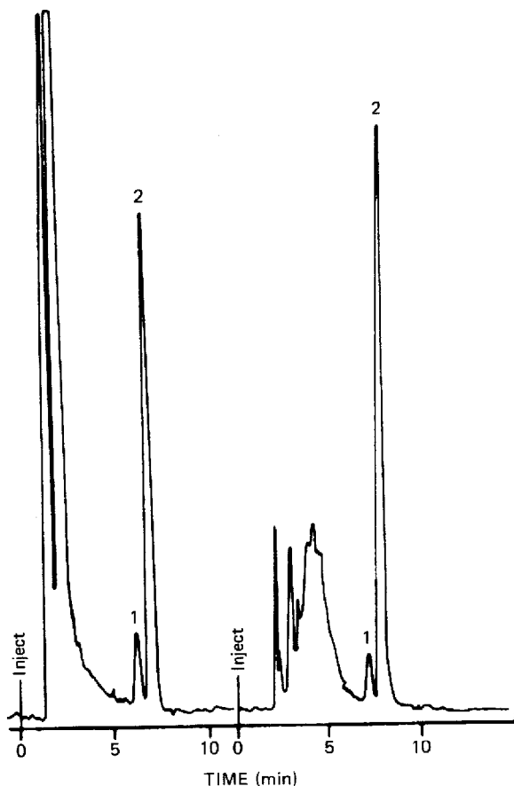
Fig. 17. Chromatogram of extracts of plasma (left) and platelets (right). Column, 10- \mu\text{m} \mu\text{Bondapak C}_{18} (30 cm \times 0.39 cm I.D.); eluent, methanol-water (98:2, v/v); flow-rate, 1.4 ml/min; detection, fluorescence (Perkin-Elmer 650-10S), \lambda_{\text{exc}} 292 nm, \lambda_{\text{em}} 325 nm. Peaks: 1 = \gamma -tocopherol; 2 = \alpha -tocopherol. From ref. 242, with permission.
